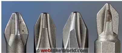
TEST: Which is the Phillips and which is the JIS? (See next photo).
