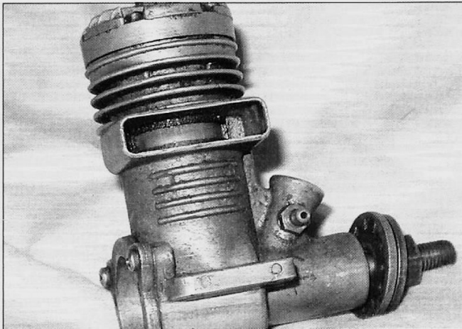
STEP 1 – Rotate the piston so the exhaust port is closed off to water entering the cylinder
