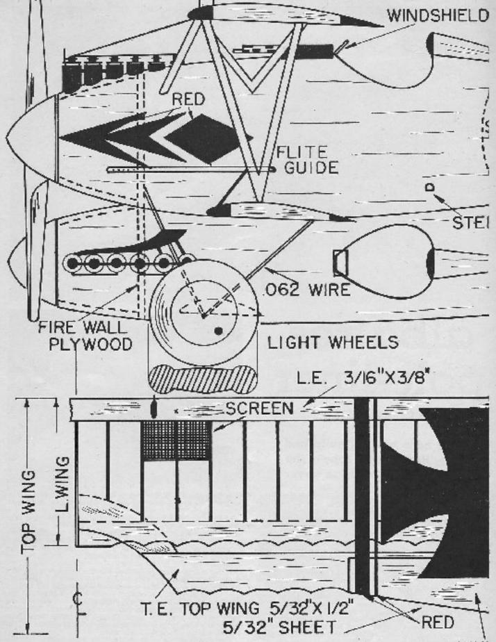
If someone wants to try this, I will loan you the magazine to copy everything you need. Construction is a hollow log type fuselage with a built up wing and sheet tail surfaces. Not much detail shown for engine mounting or other hardware. Magazine cover says Half –A power. Plans calls out Anderson Spitfire engine. The Article states routing the flying line through the flight guide (not very clear on plan) and attaching it to one of the motor mounting screws
