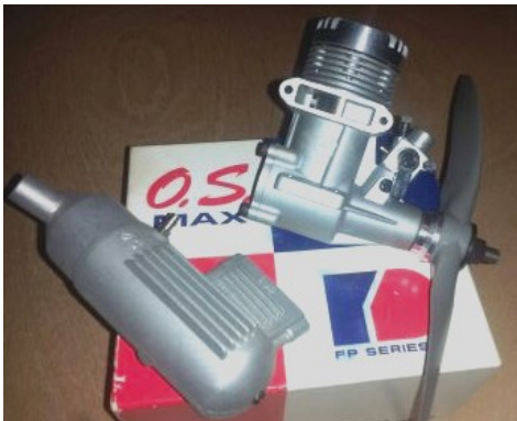
Here is our stock FP40 complete with budget carburetor and standard dustbin style muffler. What can we do to take it up a notch?
