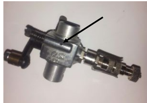
Here's the el-cheapo carb. The arrow points to the air bleed hole that hopefully lets in enough air to keep her runnin' at idle.
