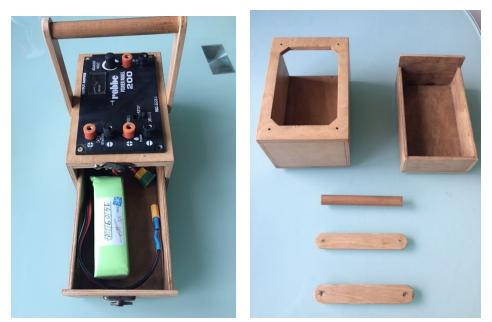
This is a little box to hold a 3S lipo and a power panel. It provides a much lighter solution for flight line use. The Lipo provides a lot of power, but there is no overdischarge protection. It should only need to be charged a few times a year.
