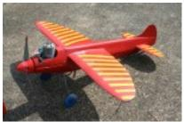
The model is very small and only has a 18" wingspan and most today are powered with .15
