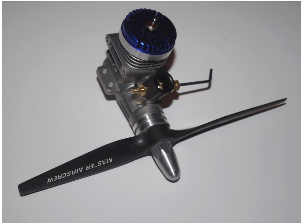
Here's an engine project I have been working on. It's a Magnum .15 set up per Dallas Sport Goodyear racing rules. The engine was the subject of the bearing article I did a couple months ago. It also has a venturi made according to the techniques in another previous *Circulator* article. The needle valve assembly is a Super Tigre style unit from RSM. The spinner nut was turned from a piece of half inch 6061 aluminum hex stock on my sherline lathe. It should be all ready for some bench runs.
