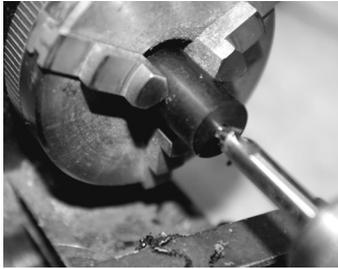
A center drill is used to mark the center for through drilling. A small diameter standard bit can be used as a substitute
