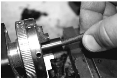
Now it's time to smooth out the interior surface. Try to control this step so you don't end up boring out your venturi by over sanding. That being said, it will take some substantial work to smooth the venturi bore. Go in steps from 220 up to 600 grit sand paper, used wet. Even finer grit will make your venturi function and look better in the end. Take your time, you need to get a feel for this process.
