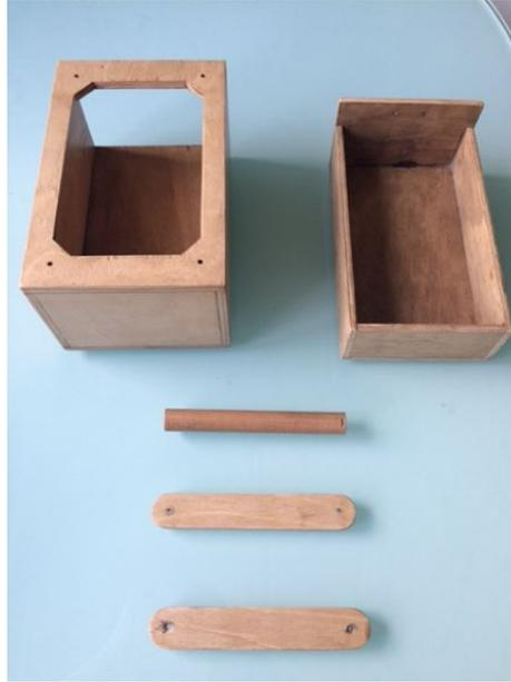
This is a little box to hold a 3S lipo and a power panel. It provides a much lighter solution for flight line use. The Lipo provides a lot of power, but there is no overdischarge protection. It should only need to be charged a few times a year.
