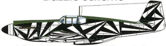
An Allison-engined Mustang was involved in a somewhat bizarre experiment in camouflage finishes during the mid-war period, when some strange concepts were being devised for camouflaging combat aircraft. It has a strange black-and-white "Dazzle" scheme on its horizontal surfaces and undersides, sometimes referred to as "confusion camouflage", but its upper surfaces are standard Olive Drab. Needless to say the application was not used in combat.
