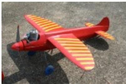
The model is very small and only has a 18" wingspan and most today are powered with .15 sized glow engines
