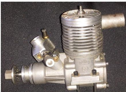
Here is my steady old MVVS .40 Q-500 racing engine that (over) powered the Albatross. Thankfully, it didn't sustain any damage during the crash. Has a Norvel .40 carburetor, the only part of a Norvel .40 engine that's good for anything. Exhaust header connects to effective tuned muffler. If anybody wants to race bi-planes, it's on!
